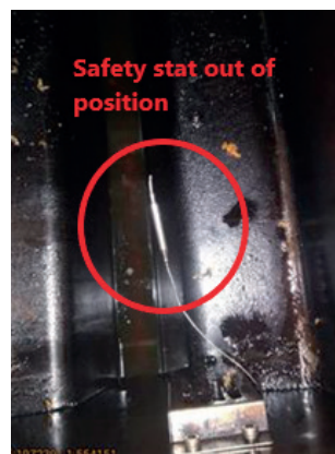
Electric fryer - Safety thermostat, broken capillary.
