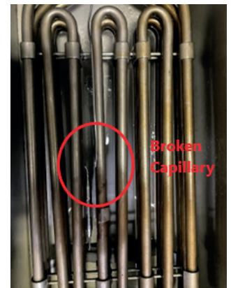
Electric fryer - Safety thermostat, broken capillary.
