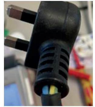
Fig 4. Exposed plug wires
