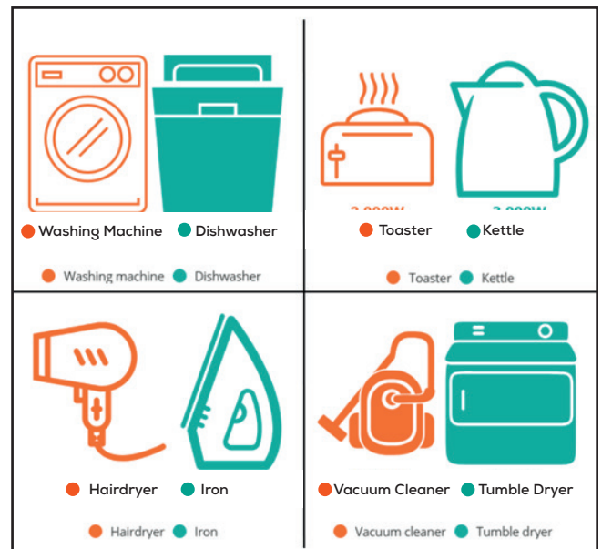
Fig 7. Example appliances that shouldn't be paired up using an extension lead.
